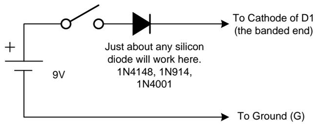
Here is a simple way to power WK for standalone applications or when the host PC does not supply a high enough voltage on the serial interface to run WK.
