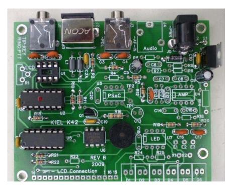
7) We can now test the keyboard and Console PIC. Plug a PS/2 keyboard into J2. Re-attach power and when power is turned on you will now hear an "R" in sidetone. When you type letters on the keyboard you will hear them sent in sidetone.
