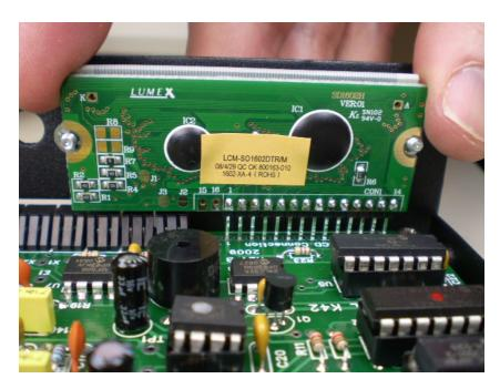
Then fold the display up into place on the threaded studs
