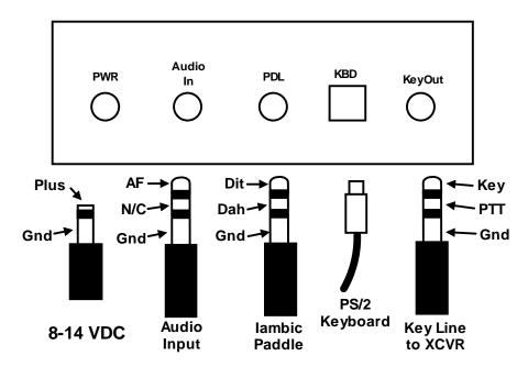
19) To install the top cover, reference the following picture. Angle the top cover and get the rear connectors to start to go into the cover. Then fold the cover down to meet the front panel and push it forward so the three 1/8 inch connectors poke out the back evenly. Install the four black 4-40 screws to hold the cover in place.
