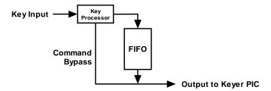
Figure 2 - Output FIFO Block Diagram
