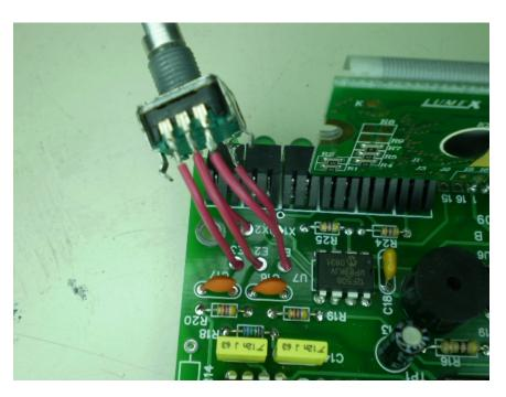
Then solder the remaining three wires: E1, E2, and E3
