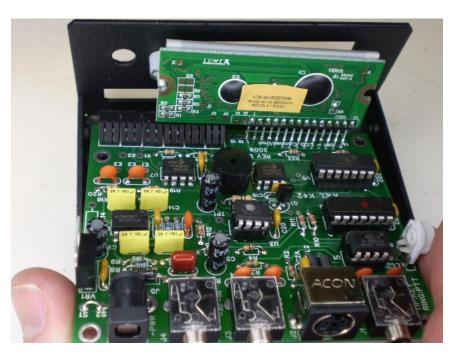
Now carefully remove the LCD display/K42 PCB assembly and solder the remaining header pins from the bottom of the K42 board. **SOLDER THE TACKED JOINTS LAST** to preserve your alignment.
