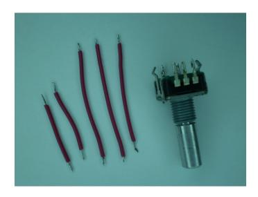
Prepare five wires, two are 1 inch long the remaining three are 2 inches long. Strip and tin both ends as shown in the picture.
