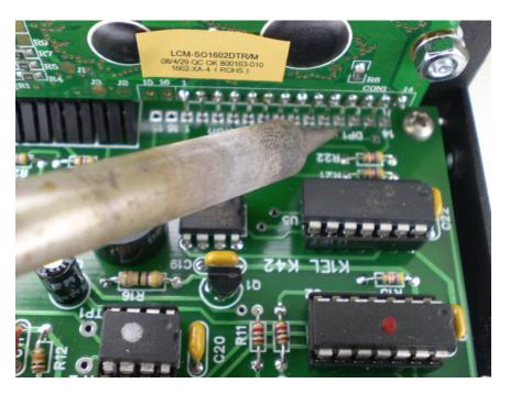
Make sure the K42 PC board is firmly seated on the enclosure standoffs and that the display is held firmly in place by the 4-40 nuts. Now very carefully sneak in with your soldering iron and tack solder two pins on the header to the K42 main board as shown. Solder the fourth pin in from each end, being careful that the barrel of your soldering iron does not come in contact with anything.
