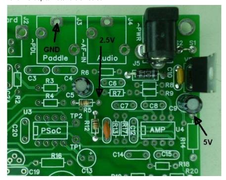
3) Once these parts are soldered in place, trim the component leads and then make up a power supply connector plug to test the board. A mate to J5 (P1) is included in the kit. Solder two wires to the connector the plus lead will go to the center pin. Wire for this cable is not provided in the kit.
