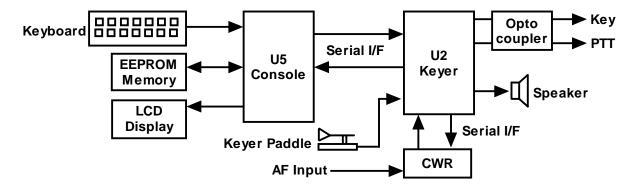
Figure 1 - K42 CW Keyboard Block Diagram
