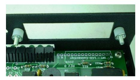
Now carefully install the display so that the header pins fit into the K42 board and the LCD mounting ears fit in place on the threaded studs. This will take a little coaxing to get into place. Please remember to handle the display on its sides so as not to damage the display's wire film ribbon cable (looks like paper).
