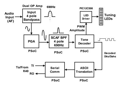
Figure 3 - K42 CW Reader Block Diagram
