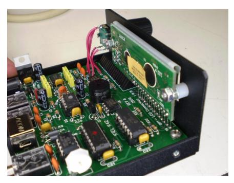
LCD Display Mounted in proper position
