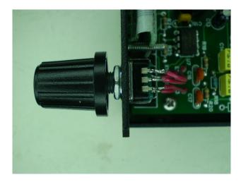
17) The encoder is mounted with one hex nut and one flat washer. The washer and nut both go on the front of the unit. Reference the picture above to see how this is done. You might want to put a spacer on the inside so the control knob will rest closer to the enclosure but that's up to you. Be careful when tightening the nut, it's easy to slip and scratch the front panel. Now attach the rotary encoder knob using a 5/64 inch Allen wrench.
