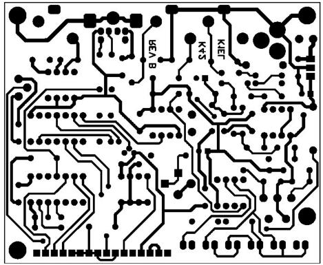
Figure 7 - K42 CW Bottom Copper
