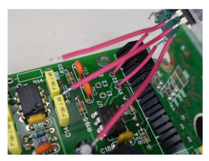
Solder in the X1 and X2 wires first
