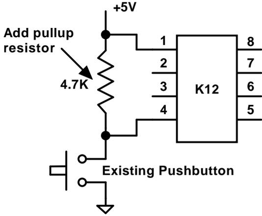
Simply solder a 4.7K 1/4 or 1/16 watt resistor between ppin pads 1 and 4 on the bottom (solder) side of the PC board.
