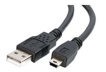
The right facing side connectors are labeled **USB** and **AUX**. The USB connector is designed to mate with a Type A to Mini-B cable. This cable is shown at left. The interface will run at USB 1.0 and 2.0 speeds but is not compatible with USB 3.0.
