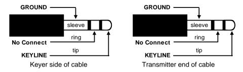
The nice thing about using a stereo connector on the keyer side is that you can easily add PTT or a second key line in the future. On the transceiver end, the key line goes to tip and ground goes to the sleeve. Make sure you disable the radio's internal keyer (if it has one) and set it up for
