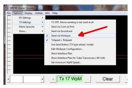
A simple WinKeyer configuration dialog box is displayed. Enter the com port number as reported by WKscan and click Save. WKmini is now active and you can set up configuration options. Select paddle Keyer Type, lambic B is most commonly used. Then if you want to use a single key port with PTT select Key Port 1 and Ptt, else select either Key Port 1 or Key Port 2 leaving Ptt off. Enable sidetone so that WKmini's debug LED will work.
