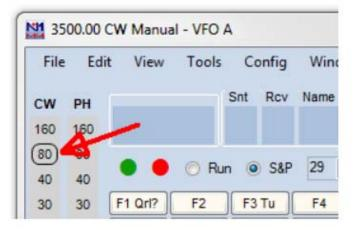
Now on the PC's keyboard enter CTL-T to put WKmini into tune mode. Cancel tune mode by entering CTL-T a second time. With tune on, your radio will be keyed to allow tuning. If you don't have a radio connected, the test LED will be lit and can be seen through the hole in the side. Now either enter CTL-K or select the CW Key Window as shown:
