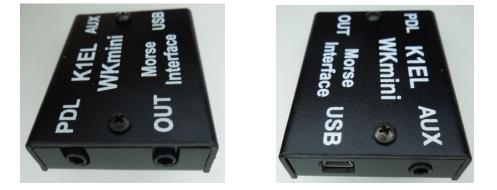
There are four connectors on WKmini, two on the left side and two on the right, The left facing connectors are labeled PDL and OUT. The PDL connector is an 1/8" stereo jack which accepts paddleset input. The paddle can be an iambic or side swiper type. A bug is not acceptable. The paddle inputs are activated when switched to common ground (GND). The paddle connector needs to be wired this way:
