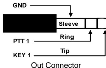
The AUX connector uses the same type connector as OUT. It provides a single switched output for KEY2. Like OUT, this output is isolated from WKmini ground and all other WKmini signals by an optically coupled solid state relay which insures a 5000V barrier. The output can switch a voltage up to +/- 60 V, keyed current up to 120 mA. The output connector wiring is shown below:
