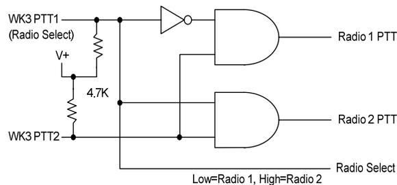
The PTT outputs on WKMINI are open collector so pull up resistors are required to generate logic high and low conditions. PTT1 will be logic zero when radio 1 is selected and logic one when radio 2 is selected.
