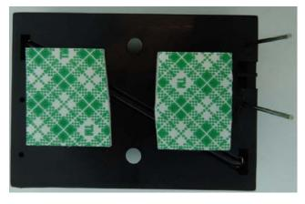
Figure 8 – Two sided foam pieces on bottom of battery holder.
