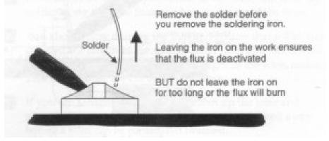
Fig C3 - Remove the solder
