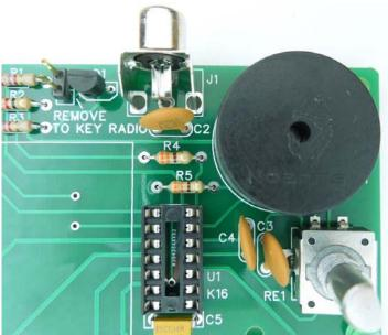
Figure 7 – RCA jack and Encoder installed
