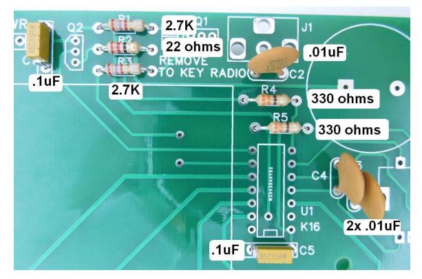
Figure 5 - Resistors and capacitors installed
