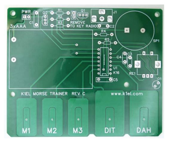
Figure 2 – Morse Tutor PC Board (MTB) before assembly
