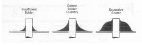
Fig. C4 - Solder quantity comparison
