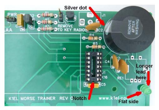
Figure 6 – Socket, 2 pin headers, Q1, Q2, speaker, and LED installed
