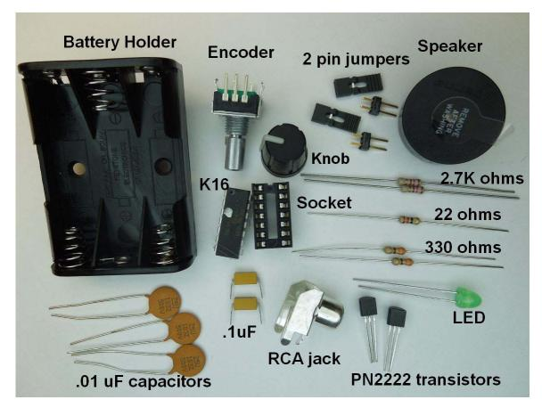
Figure 3 - MTB component identification
