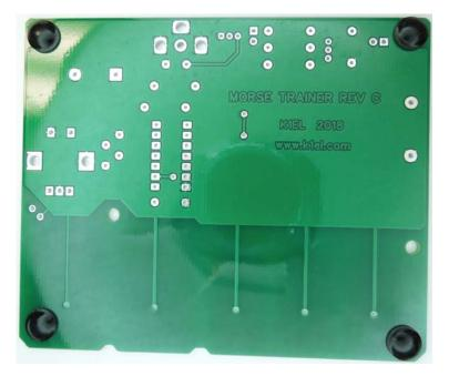
Figure 4 – Rubber feet in place
