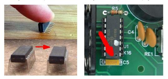
Figure 9 – Straighten leads on U1, then install in socket
