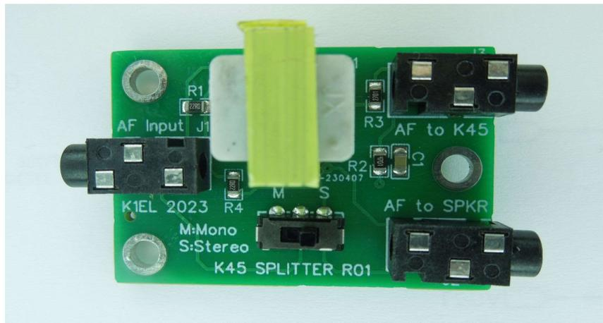
Figure 1 – K45 Audio Splitter board
