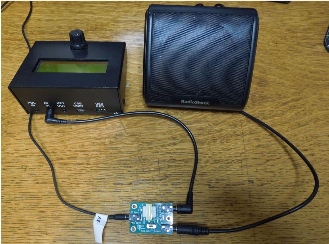
Figure 3 – K45 Audio Splitter cabling example
