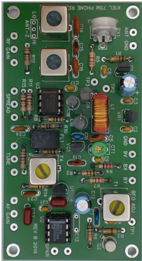
Figure 1 – Assembled AMR75 Board
